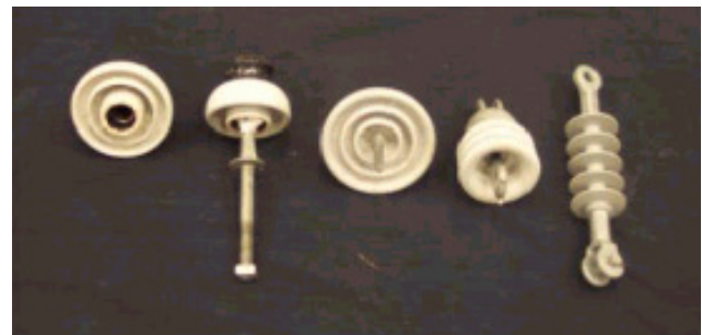
Fig. 1. Tested insulators, from the left: ANSI 55-4, ANSI 55-3, ANSI 52-1, ANSI 52-9, 15 kV Polymer Suspension.
