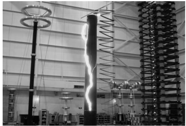
Fig. 4. The 35 kV porcelain pin insulator plus fiberglass pole, the tested pole length is 8 feet. The discharge developed on the surface of insulator and the pole
