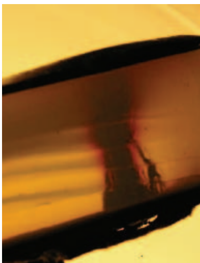
Fig. 5. Example of treeing in failed cable
