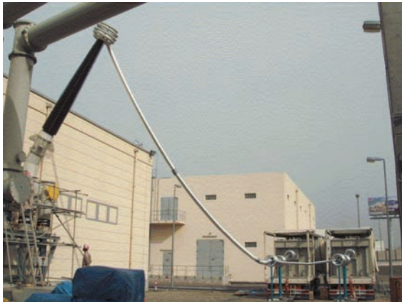
Fig. 4a. Parallel setup of two resonant test systems for testing an 11-km 380-kV cable installation
